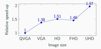
The higher resolution is, the higher relative speed-up is (with speed-up on QVGA taken as 1.0).
